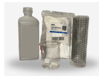
Fig. 5. TiO 2 anatase nanopowder, IPA precursor, mesh substrate. Image taken by student researcher, Shanza Sami.
